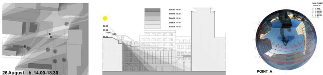
Fig. 2 Solar input analysis by means of architectural survey and Solar Pathfinder™
