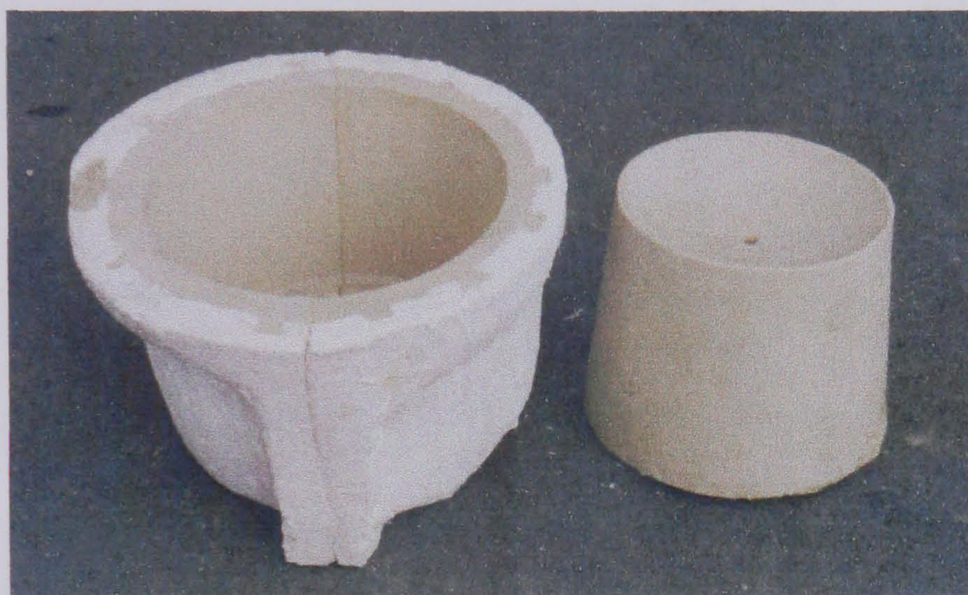
Fig. 6 The Hot-Melt Vinyl rubber cases. The left one was used to cast the exterior wall surface and the right, the interior.
