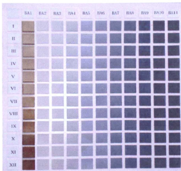
Fig.4.10. The heated row of sample BA1 highlighted to show that white inclined to go to ochre colour when heat was applied at 70°C for 10".
