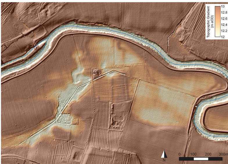
Figure 4. Lidar image with the pale grey/tan areas mapping the approximate line of the prehistoric palaeochannel (B. Pears).
