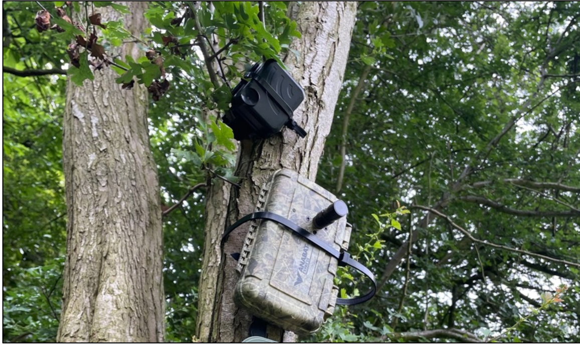
Figure 1.4: A commercial (bottom) and open source (top) acoustic detector deployed in the field, targeting bats.
