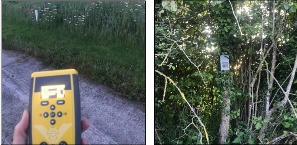
Hand-held detector on a transect survey versus passive detector on an automated survey
