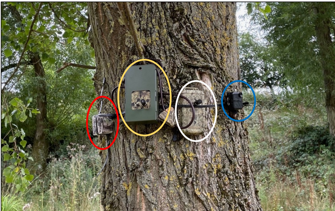
Figure 4.2: Passive acoustic bat detectors: Anabat Swift (highlighted in yellow), Anabat Express (highlighted in white), AudioMoth in proprietary case (highlighted in blue), and AudioMoth in junction box case (highlighted in red).
