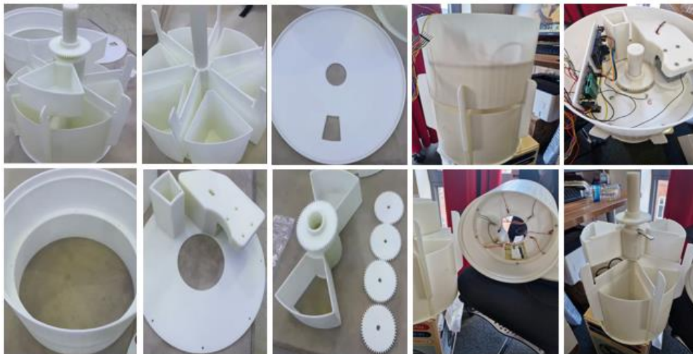
Figure 5. Different images show the 3D-printed parts of the physical bin's design
