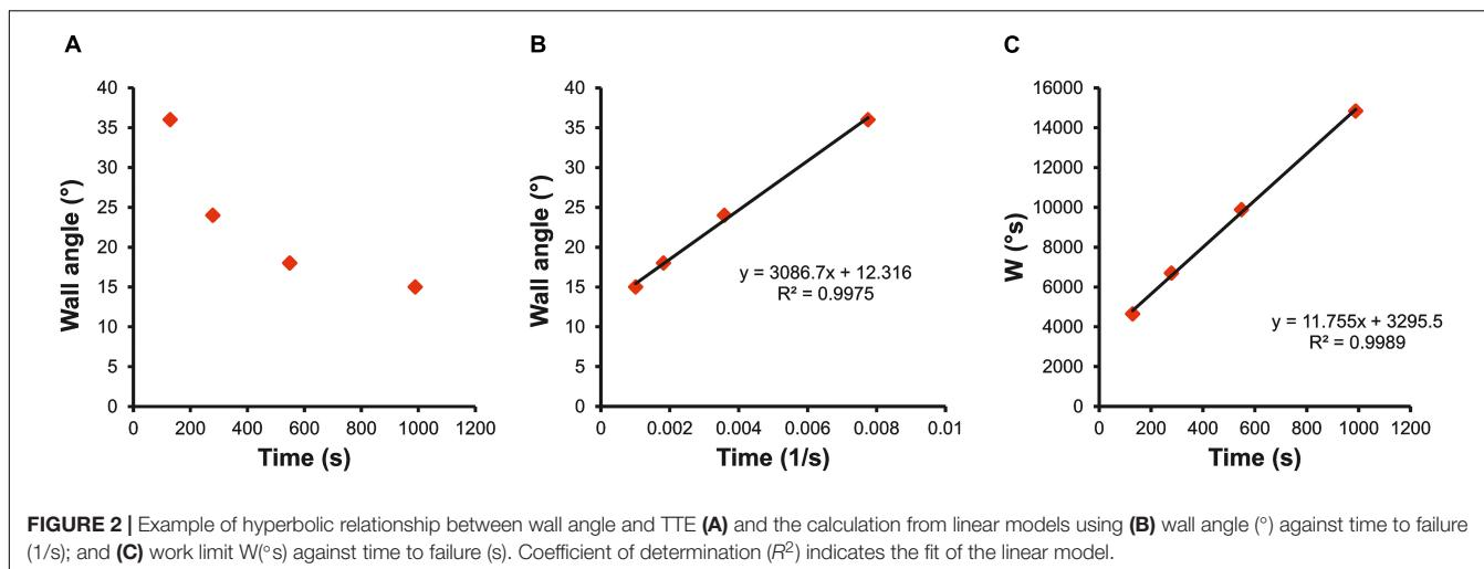
**FIGURE 2** | Example of hyperbolic relationship between wall angle and TTE (A) and the calculation from linear models using (B) wall angle (°) against time to failure (1/s); and (C) work limit W(°s) against time to failure (s). Coefficient of determination ( $R^2$ ) indicates the fit of the linear model.
