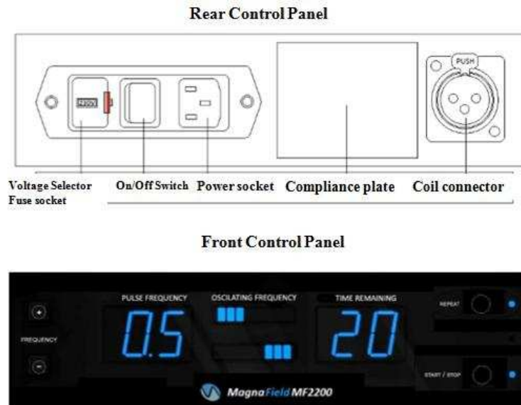
Figure 2 The front and rear control panels
