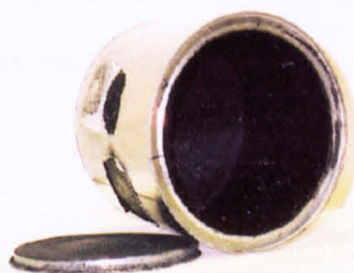
Fig. 1.10 Pinhole camera with blackened interior
