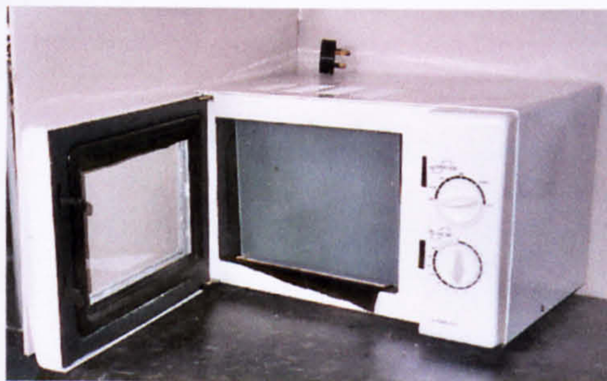
Fig. 3.15 Etched glass screen set back behind plain glass in microwave
