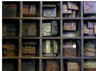
Trays of pantograph dies at Graziani, Napoli
