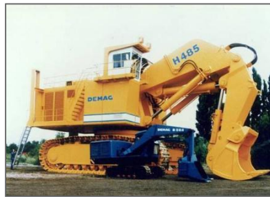
1986 Worldwide largest hydraulic mining shovel (500 t) – H 485
