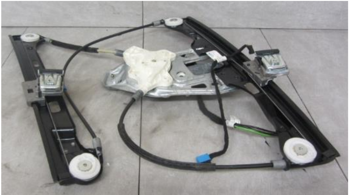
Figure 5-44 Example of a Cable Pull (dajo Autoteile, 2013)
